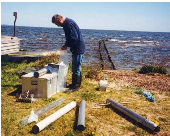
Figure 3.2. Drill corer and PVC tube (left) and core sampling at the Reed zone east of Mönkebude (right).
