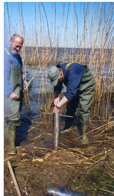
Figure 3.2. Drill corer and PVC tube (left) and core sampling at the Reed zone east of Mönkebude (right).
