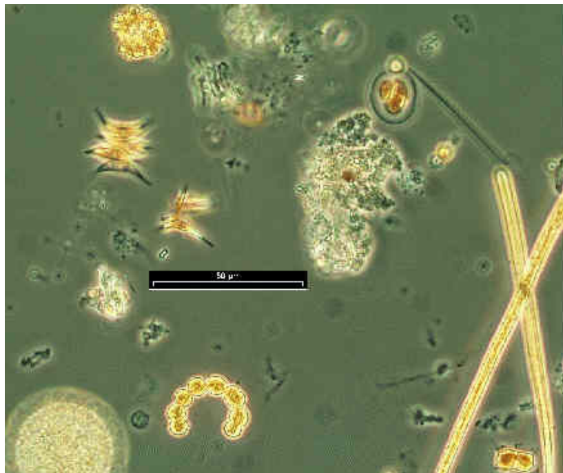
Figure 4.19. Inverted microscope picture showing the dominance of organic components within the Oder Lagoon suspended particulate matter.
