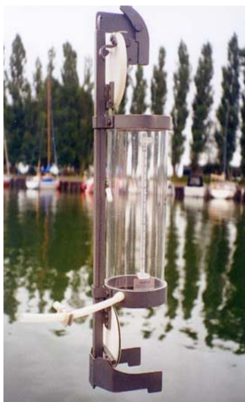
Figure 3.5. Water sampler used for taking water sample at particular depths.
