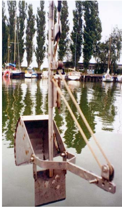
Figure 3.1. Grab sediment sampler used for taking offshore sediment samples.
