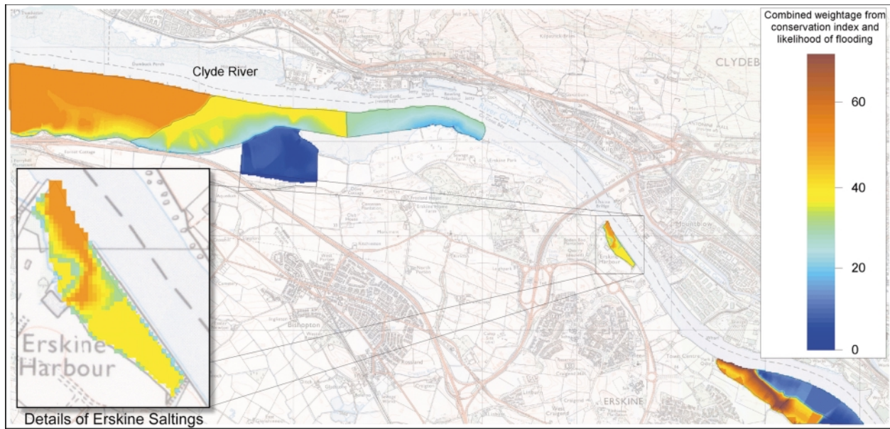
Fig. 4. Combined flood risk and ecological evaluation weighting showing ecological ‘value’ of conservation areas lost by flooding to 6.0 m above MHT. Ordnance Survey base map reproduced by permission. Crown Copyright Approved.
