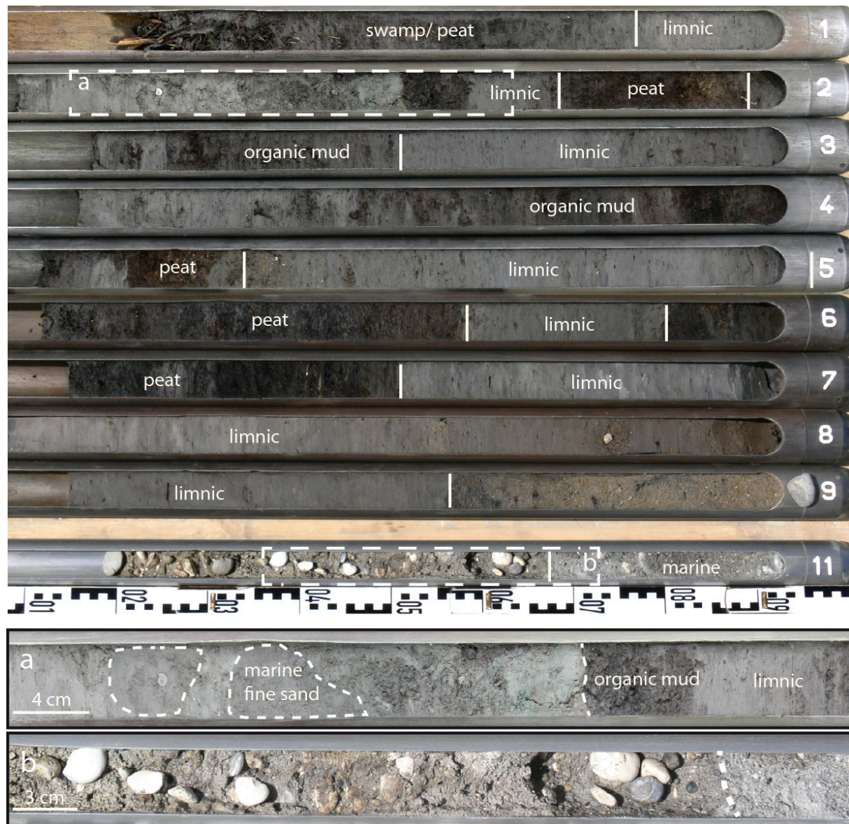
Figure 4: Simplified facies profile of vibracore LIX 7. Allochthonous high-energy tsunami deposits are marked with white borders.
