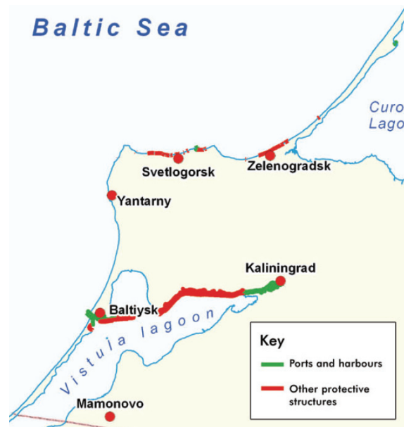
Figure 4: Map showing artificial structures along Kaliningrad coasts, built to provide local shoreline stabilization (from Gilbert 2009). The protective measures along the northern coastal segment near Svetlogorsk and Zelenogradsk result in problematic sand deficits along the Curonian Spit all the way to Klaipeda and beyond (see chapt. 8).
