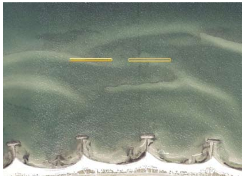
Fig. 2: Example with two submerged breakwaters (alternative 2) (source: Kliucininkaite 2011)
