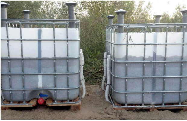
Photo VI Pilot installation of a Red Bed System, photo: A. Kupczyk.
