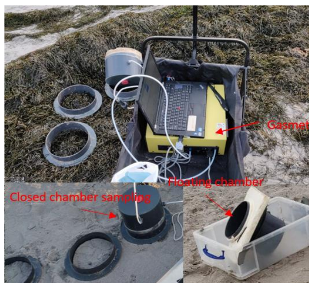
Figure 2.2.3. Gaset machine in use at Køge beach; closed chambers with tubes for the air flow to Gaset are seen.
