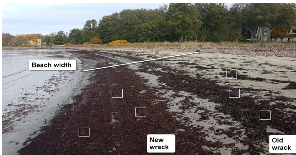
Figure 2.2.1. Example of placement of biomass samples (3 frames from fresh material, 3 frames from older material). Beach wrack was estimated and litter from the water's edge to the back of the beach (in beach width) was collected along the 100 m beach length (Kakumäe beach, 15.10.2019; T. Möller).
