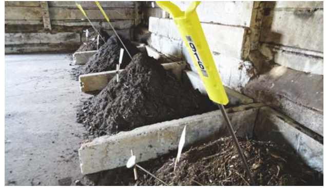
Compost piles with wireless temperature probes at the Hanseatische Umwelt CAM GmbH facilities.
